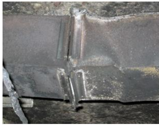
Significant damage on a smoke control duct – 30 minute fire resistance
